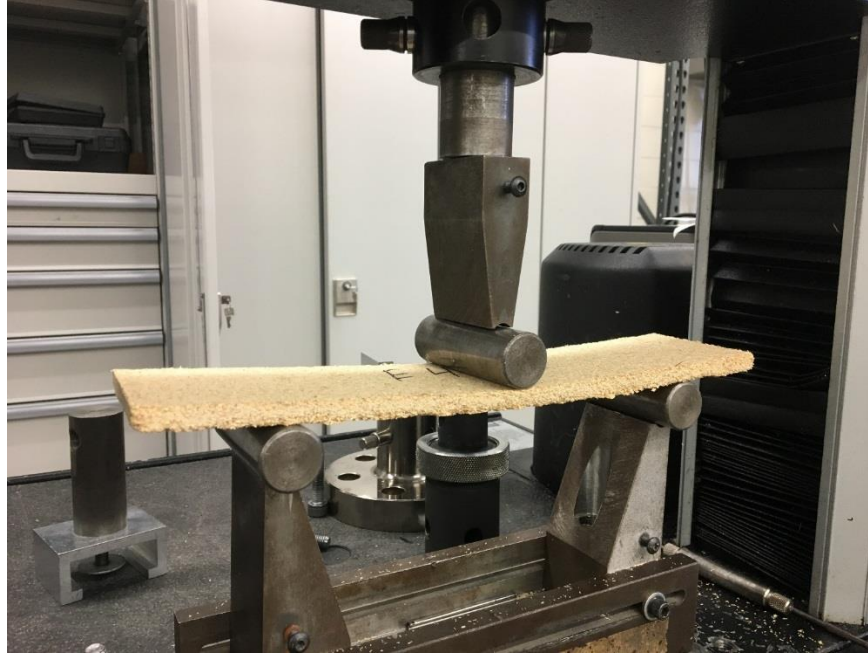
Figure 10: Three-point static bending as prescribed by ASTM D1037 being conducted on an Instron load frame model 5567
