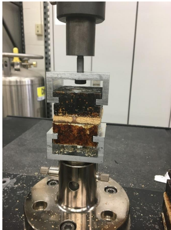
Figure 11: Internal bond blocks loaded into Instron load frame model 5576
