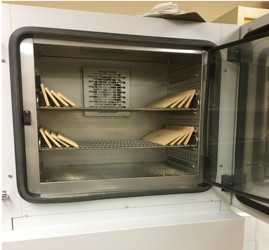
Figure 9: Linear expansion setup in the Binder Humidity Chamber model KBF 115-UL
