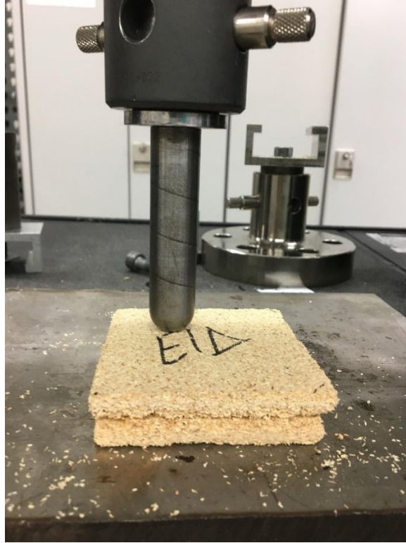
Figure 13: Janka-ball hardness indenter test pre-run on the Instron load frame
