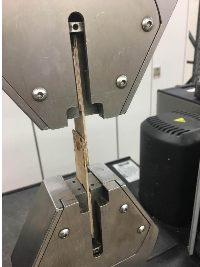
Figure 5: Lap Shear sample being tested in Inston load frame model 5567
