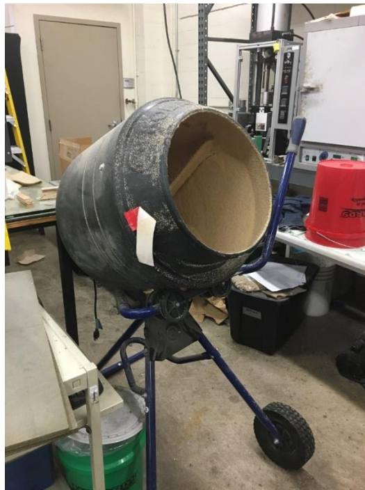
Figure 6: Kobalt cement mixer used to mix resin and wood flour
