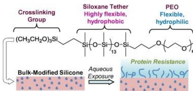
Figure 1.7. Chemical structure of PEO-silane amphiphile (n = 3, 8, and 16) and surface reconstruction of bulk-modified silicone coating with PEO-silane amphiphile. Reproduced from reference 95
