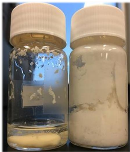
Figure 2.2. Carbinol-isocyanate (left) and silanol-isocyanate (right) product appearance
