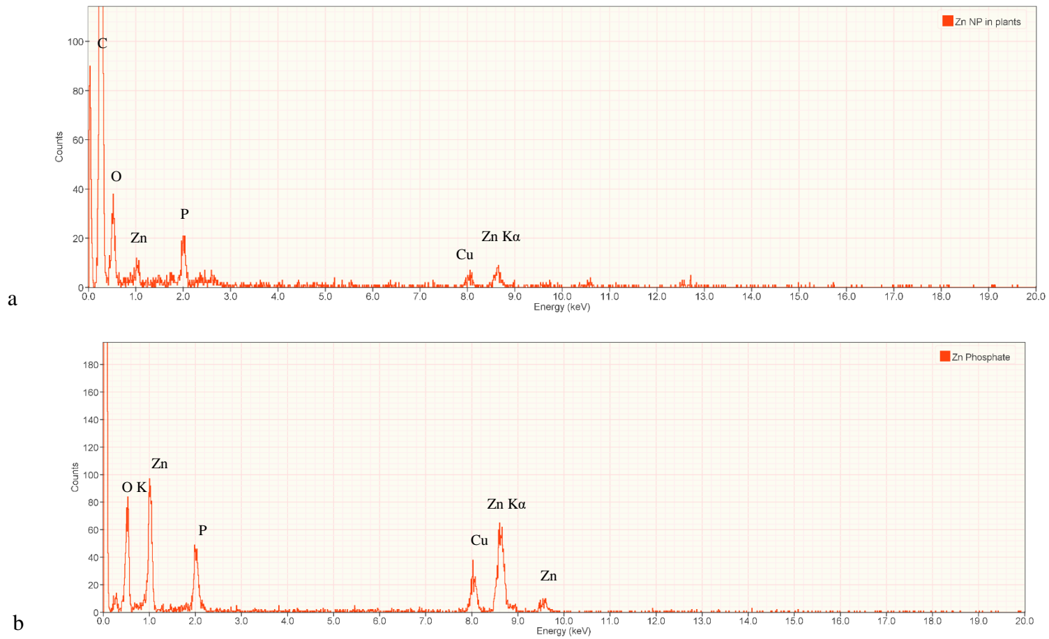
Figure 3.6. EDS Spectra of different Zn compounds (a) Zn NP in plant roots, (b) Zn phosphate, (c) Zn phytate (d) bare ZnO NP, and (e) overlay of Zn NP in plants, Zn phosphate, and Zn phytate spectra
