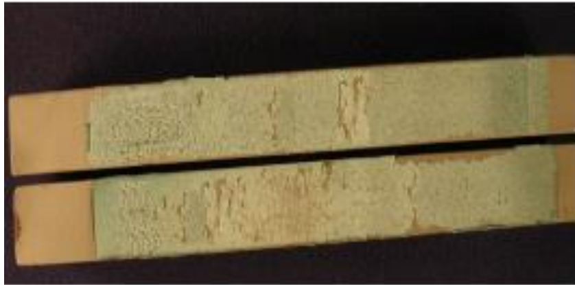
Figure 2.4. Failure surface of ABMJs under loading (Hafiz et al., 2010)
