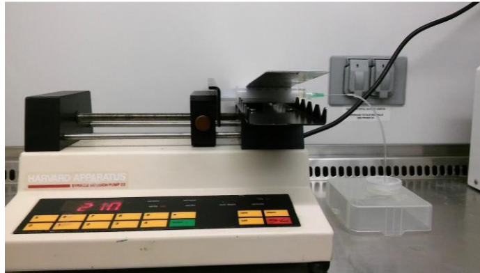
Figure 36. Experimental setup, where liquid media was flowed over a mature S. aureus biofilm grown in a small petri dish via a syringe pump.
