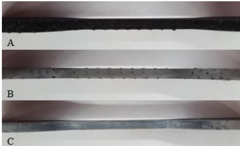
Figure 4.8: Removal of supports and surface effects. A) Supports removed, B) sanded with 60 grit paper, and C) sanded with 600 grit paper
