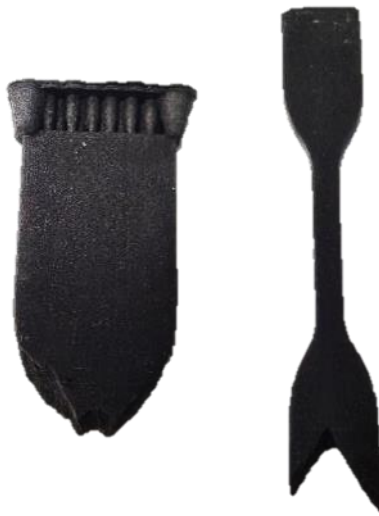
Figure 5.18: Examples of CF50-90 print failures.
