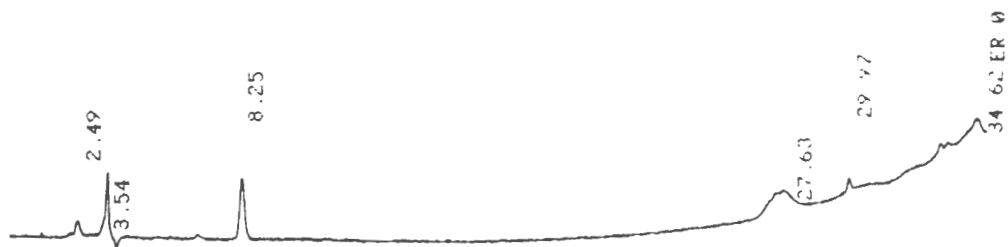
Figure 26. Chromatogram of aqueous phase speciation at 8 h in sterile topsoil.
