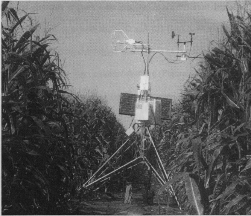
Figure A4. Weather station with complete eddy covariance system, in experimental site, Fairmount, ND.
