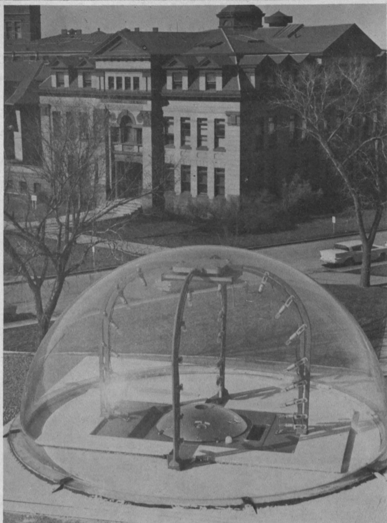
No, it's not a flying saucer. Inside this glass dome atop the library rests a camera which photographs the horizon and weather conditions each half minute. Originally set up in 1958 as part of a two-year project for the International Geophysical Year, the strange-looking device is still operating, said H. Dean Stallings, librarian. A man must change the film each two weeks.
