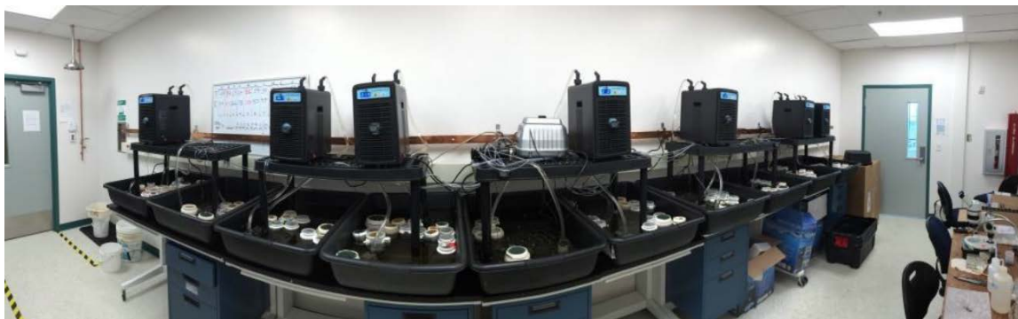
Figure 5.2. Rearing set-up in 2015 with treatments ranging from 6-29 °C. The ten black tubs (aquaria) containing floating rearing cups represent the treatments. Note the black aquarium chillers above seven of the treatments; three others were heated. The aerator is the silver pump in the center, with airline tubing running to each tub. Larger diameter hoses and a pump circulate water between each tub and its chiller in the seven cooler treatments.
