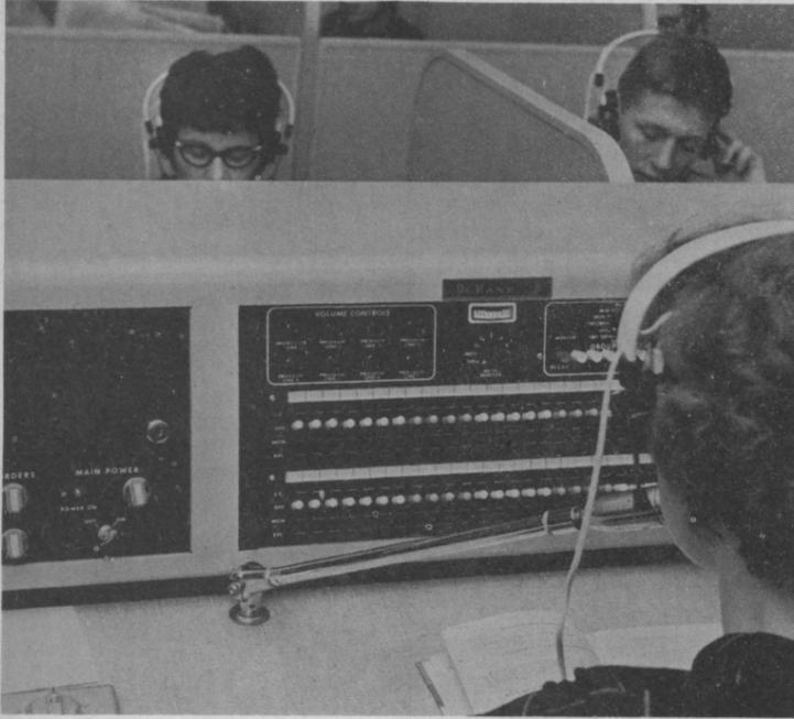
By means of new equipment installed in the foreign language laboratory at North Dakota State University, 36 students at a time can receive a form of "private tutoring" involving programmed tapes and a monitoring instructor. The new equipment is capable of programming four different languages simultaneously.
