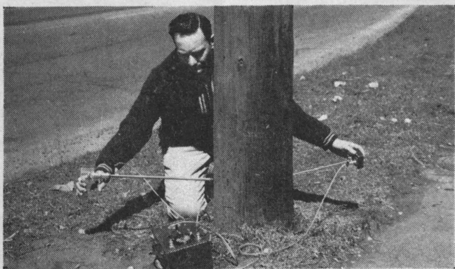
3. Transistorized circuitry was designed. And a Sonic Pole Tester was built and tested.
