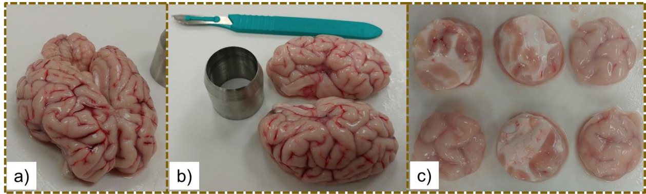
Figure 10. Sample preparation and experimental setup for an in-vitro unconfined compression test: (a) fresh animal brain and the cutting tool, (b) separating two hemispheres for cutting, (c) circular cutting tool used to extract cylindrical brain samples.
