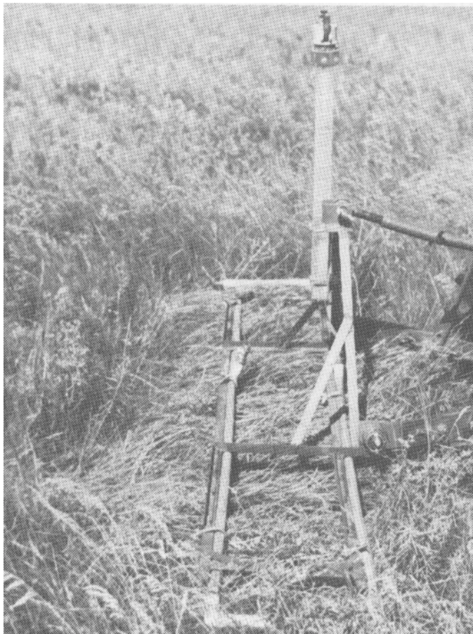
Figure 3. The wick applicator showing the double-bar frame and the sealed reservoir from the rear view (above), and the side view (below) showing that leafy spurge is treated by both the front and back wicks.
