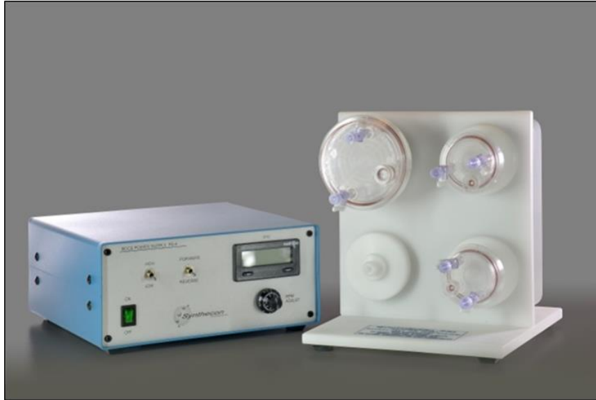
Figure 10: Synthecon Rotary Cell Culture System that produces 3D cultures.
