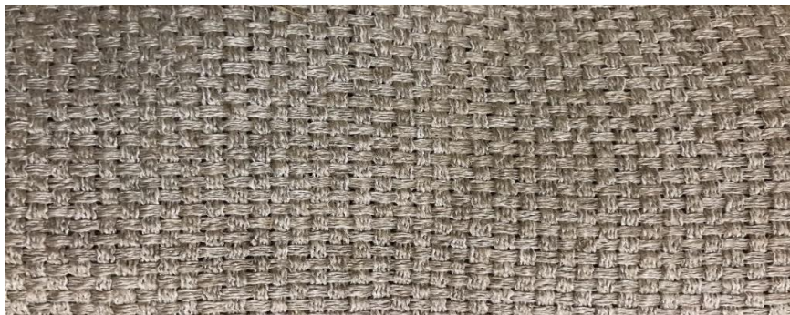
Figure 10: Woven mat of the flax fibers (Plain weave).
