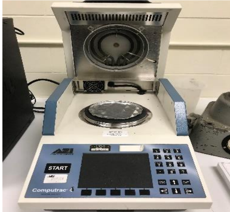
Figure 8: Moisture analyzer to measure the initial moisture content of the non-woven flax fiber mat.
