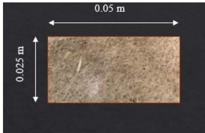
Figure 7: Non-woven flax fiber mat before the immersion into the distilled water.
