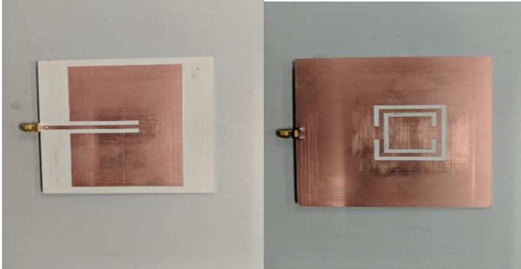
Figure 6. Fabricated dual-band CSRR patch antenna: (a) top layer and (b) bottom layer
