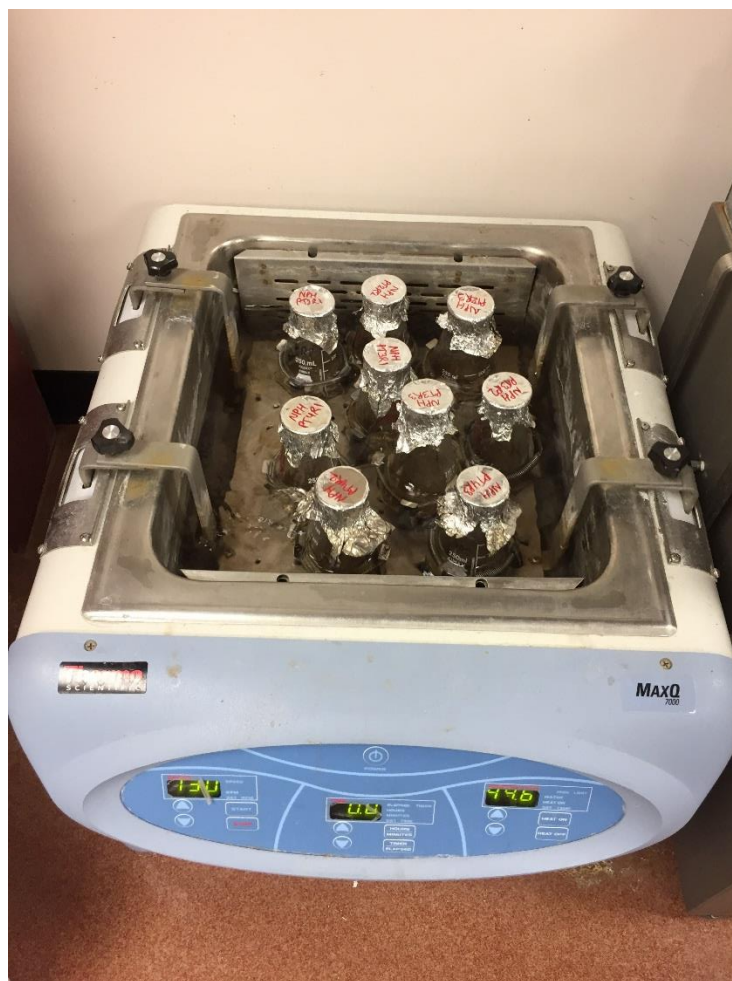
Figure A7. Hydrolysis setup in water bath
