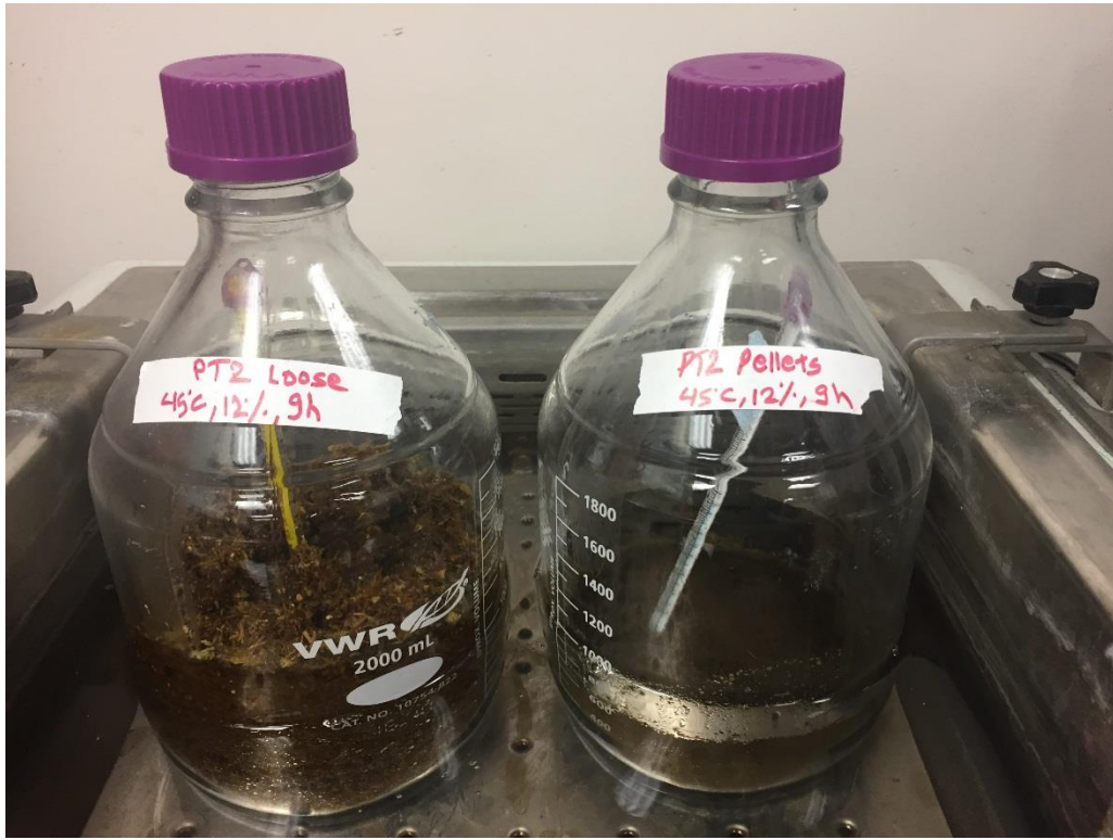
Figure A3. Pretreatment setup of loose and pelleted biomass in a water bath
