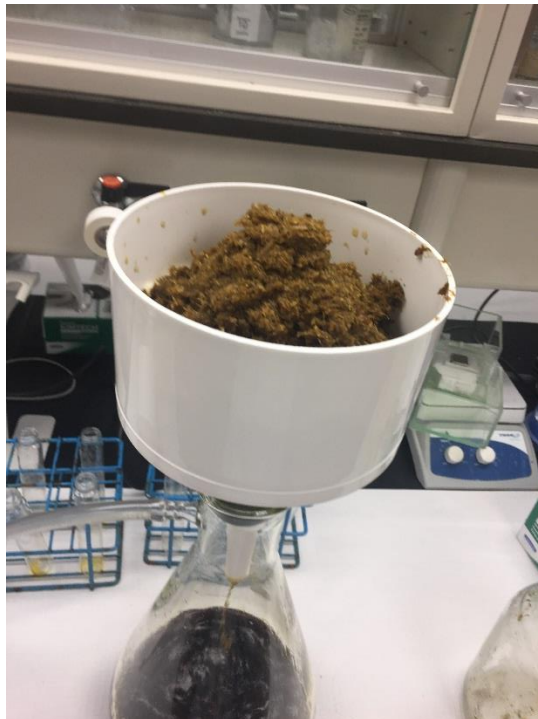
Figure A4. Washing of pretreated loose biomass
