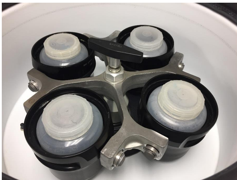
Figure A5. Washing of pretreated pelleted biomass in centrifuge
