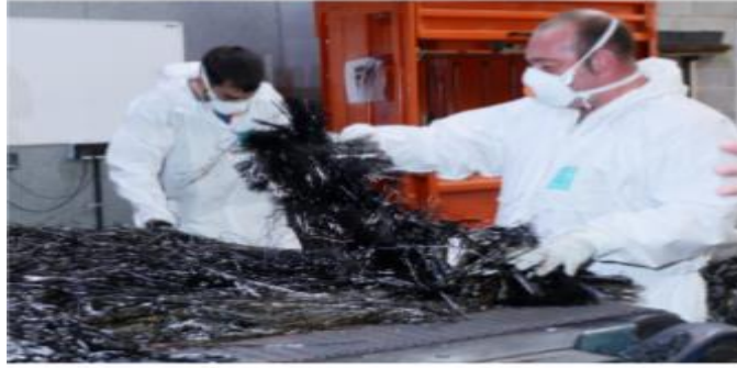
Figure 4: Feeding reclaimed carbon fiber to the furnace (Holmes, 2018)
