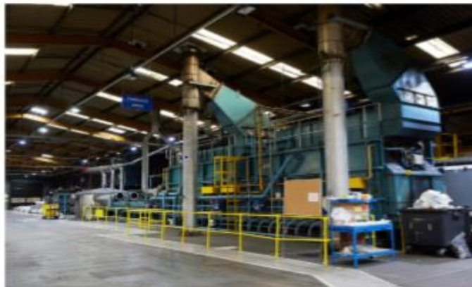
Figure 3: Fiber recovery through pyrolysis process (Holmes, 2018).
