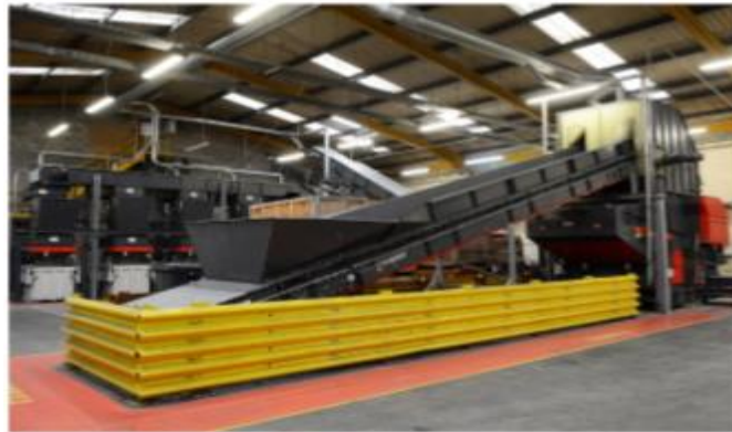
Figure 2: Carbon fiber reclamation by shredding (Holmes, 2018).
