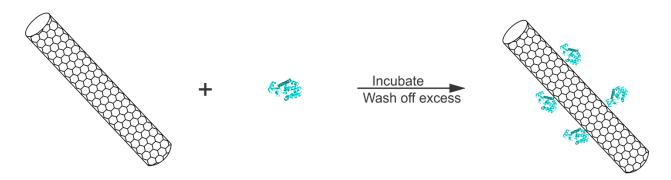
Figure 5.1. Scheme for CNT-T4L complex formation.
