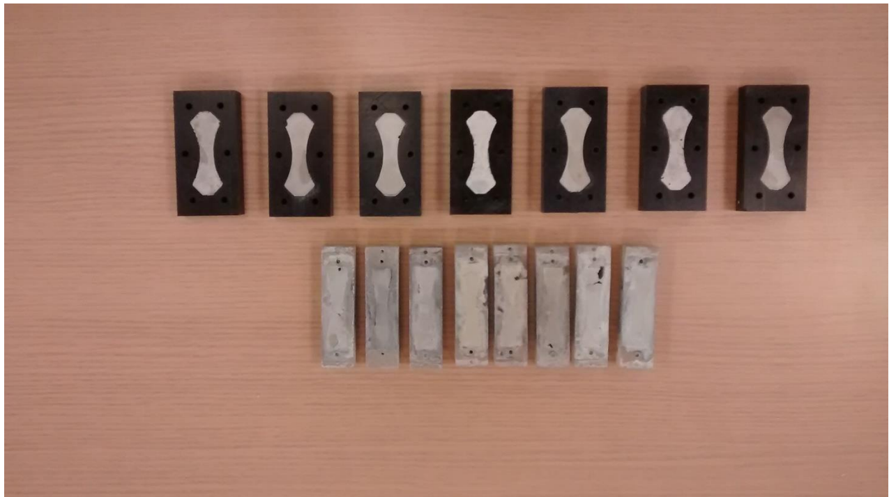
Figure 29. Paste samples in PVC molds (black), and 3D printed molds (white)
