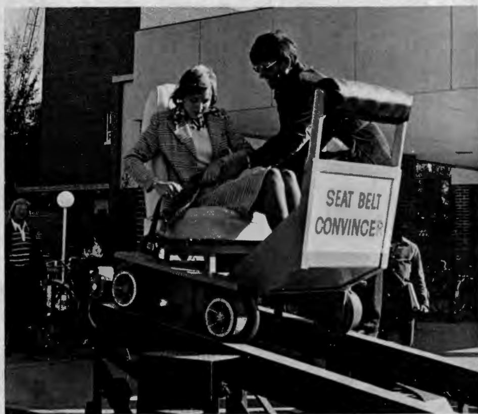
WDAY reporter Claudia Danovic, the only female to try the "convincer" during its visit to the SU campus Monday morning, is here strapped in for a ride. The device simulates a seven-mile-per-hour crash, and as the name implies, does a fairly good job of convincing people to use their seat belts. (Photo by Tom Pritchard)
