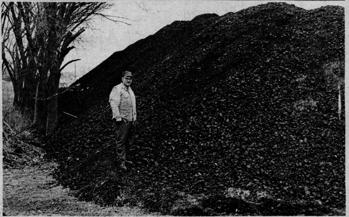
Powerplant Chief Engineer Richard Lingle shows off one of the coal piles SU has built up as a hedge against sudden coal strikes. The 1700 tons in this pile would last only 12 to 14 days. (Photo by Steve Sobczak)
