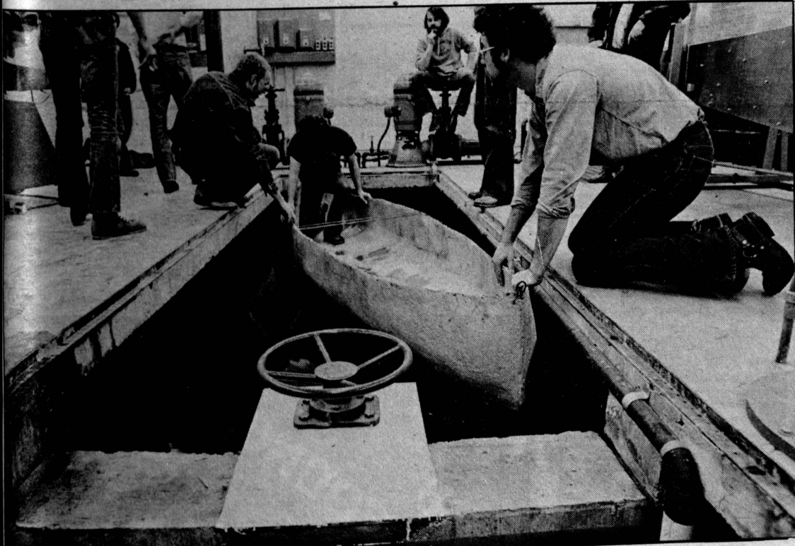
Weighing in at 220 pounds, this is the American Society of Civil Engineers concrete canoe, all 14 feet of it. Built with special guidelines for racing, the canoe will be hauled to Kansas this weekend to compete in a ASCE concrete canoe race. Members of the SU Student Chapter of ASCE are shown testing the canoe before finishing touches are added. (Photo by Jerry Anderson)
