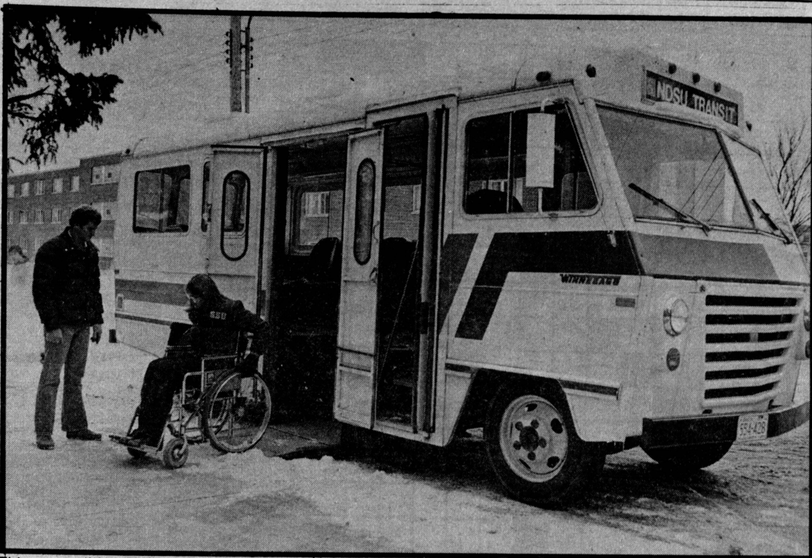
This re-conditioned Winnebago bus is part of the continuing effort at NDSU to provide handicapped student accessibility to its classes. Demonstrating the hydraulic lift are Patty Uhrich, a senior in food and nutrition and Wayne Montgomery, a graduate student in guidance.
