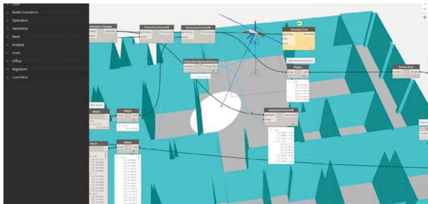
Figure 1.2 - The Dynamo interface gathering walls from Revit and testing operations with the camera component.
