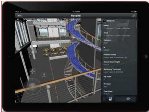
Figure 15 - BIM Glue Mobile App The Glue mobile app gives viewers the ability to view all elements associated with a model. It has all the functionalities of the desktop version, but gives the added ability to take the model virtually anywhere. It allows users to view and update model information - even in the field.
