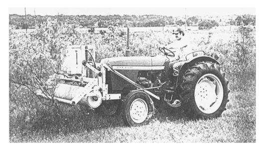
A herbicide solution is applied to small honey mesquite trees with an experimental applicator. The herbicide is wiped on by the carpeted surface of the rotating cylinder mounted in front of the tractor.
