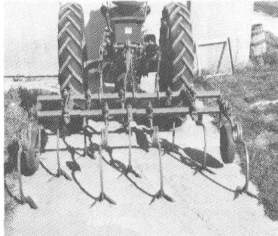
Figure 5. Duckfoot cultivator with sweeps mounted on three gangs.
