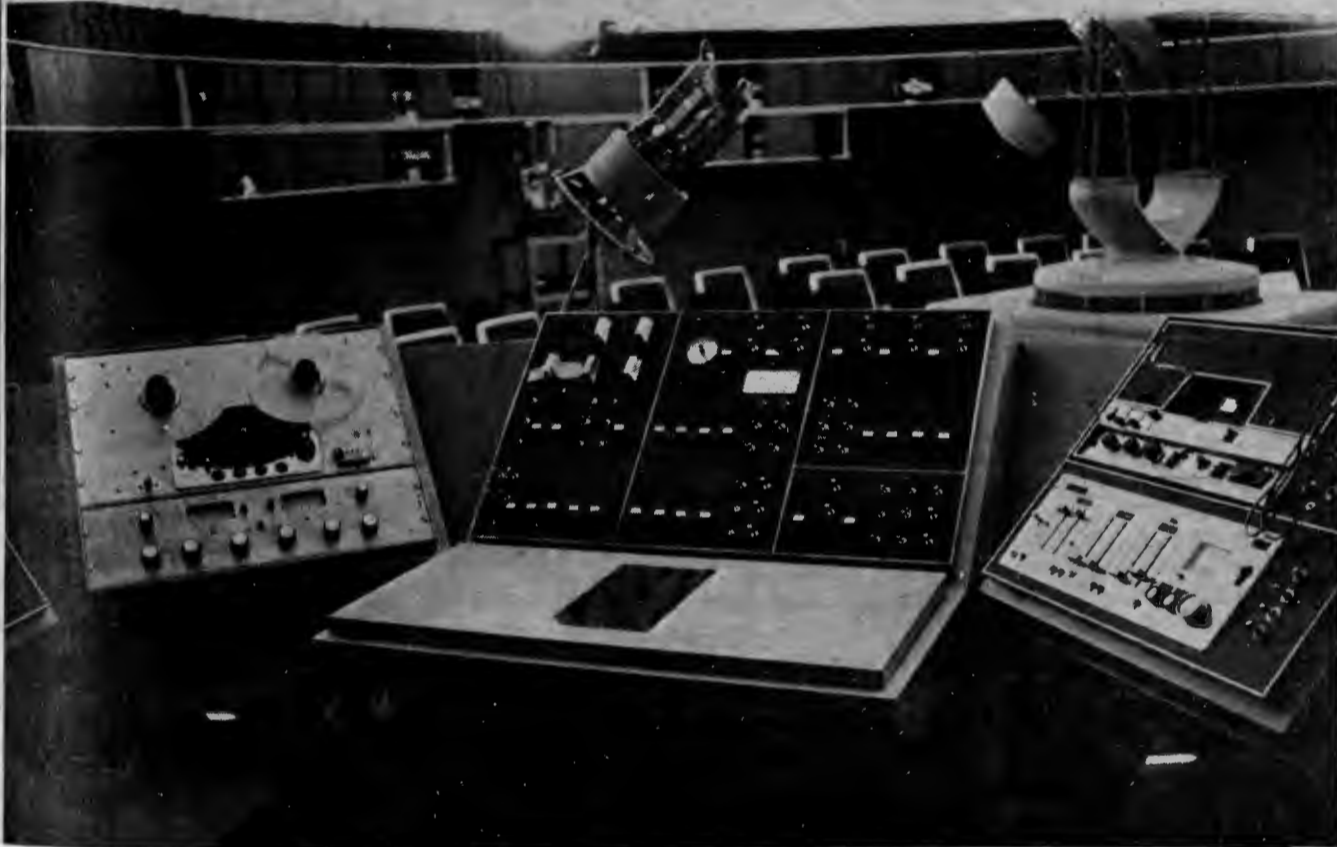
The MSU Planetarium is controlled by this console, which can control intensity, swings and tilts of the Earth's axis and other functions. (Photo by Linda Walen)
