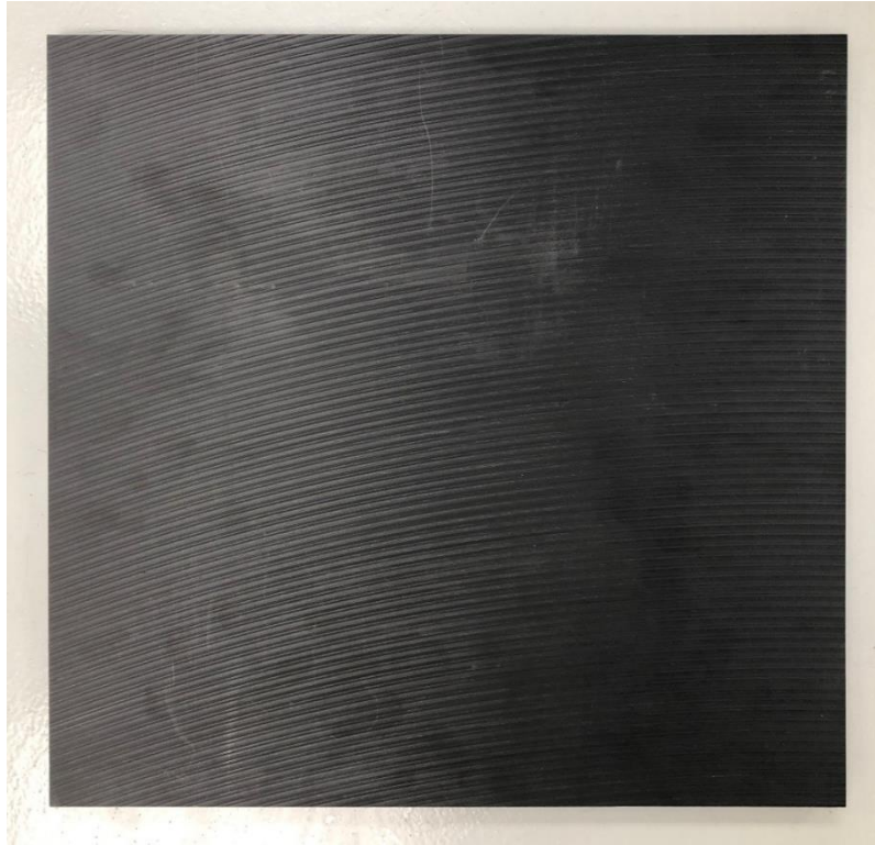
Figure 2.1. Photograph of Polycarbonate Test Sample Figure Note: The Circular Pattern on the Sample Surface is the Machining Tool Marks Generated During Production
