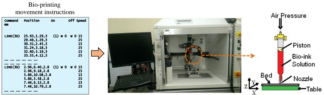
Figure 43. Micro-nozzle bio-additive material deposition system.
