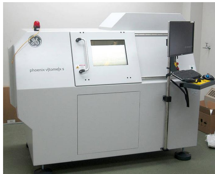
Fig. A.3. MicroCT: GE vtomex s
