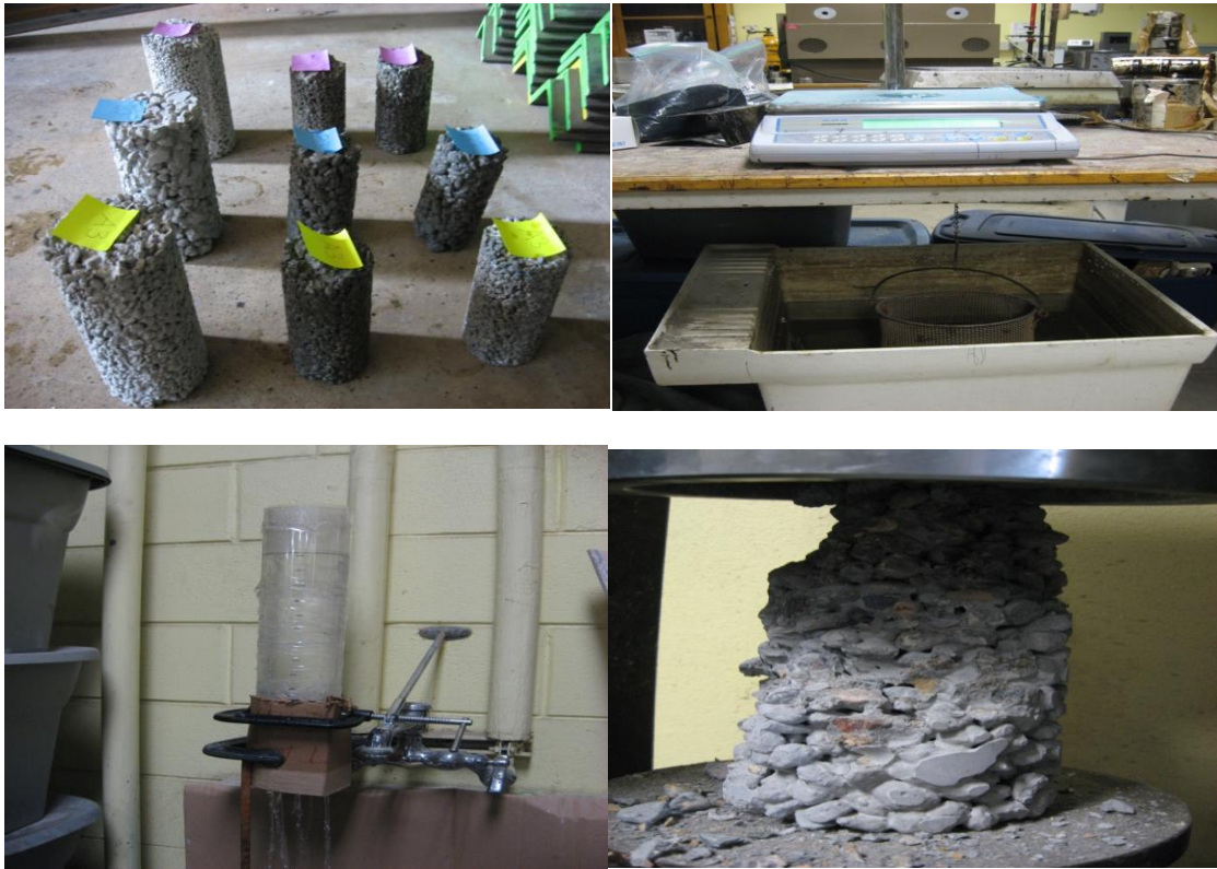
Fig. A.1. (clockwise) Batch of fiber reinforced pervious concrete samples, void ratio test, compressive strength test, permeability test
