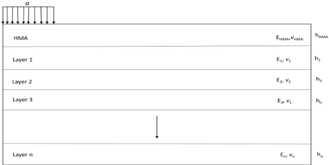
Figure 23. Flexible pavement cross-section
