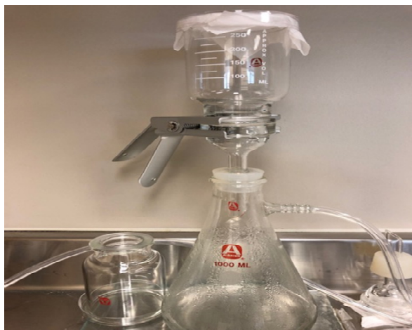
Figure 2.1. Vacuum filtration setup that we used in our project.
