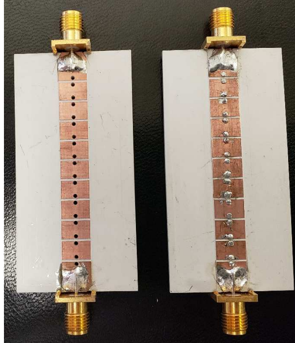
Figure 19. Prototype of the unit cell design for the open cavity case (left) and the copper via case (right).
