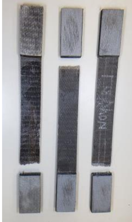
Figure 7: Fracture samples after fatigue testing.
