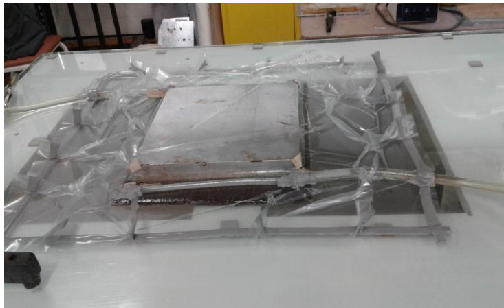
Figure 2: Vacuum assisted resin transfer molding to make composite panel [0] 12 .
