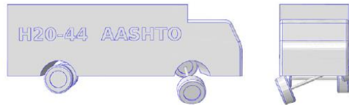
(e) Mode 5 \rightarrow f_5 = 9.016 Hz
