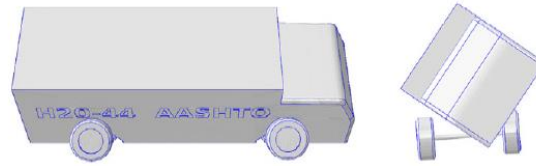
(a) Mode 1 \rightarrow f_1 = 0.927 Hz
