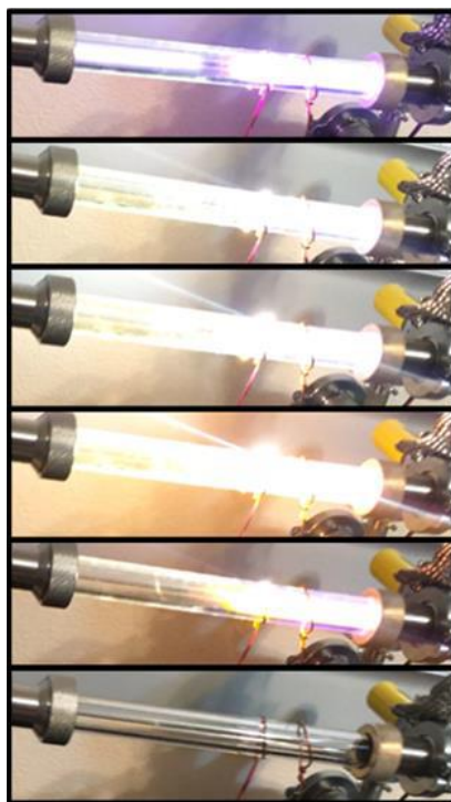
Figure 5.20. Frame Sequence of Plasma Piercing the Reactor Tube Wall at High Power (200 W).
