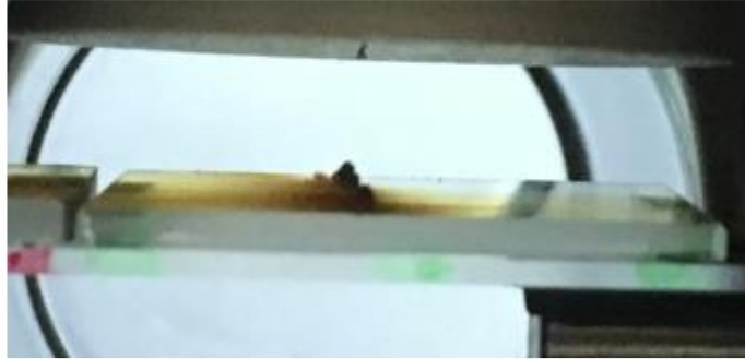
Figure 8.6. Impaction Sample Collection Through Viewport.
