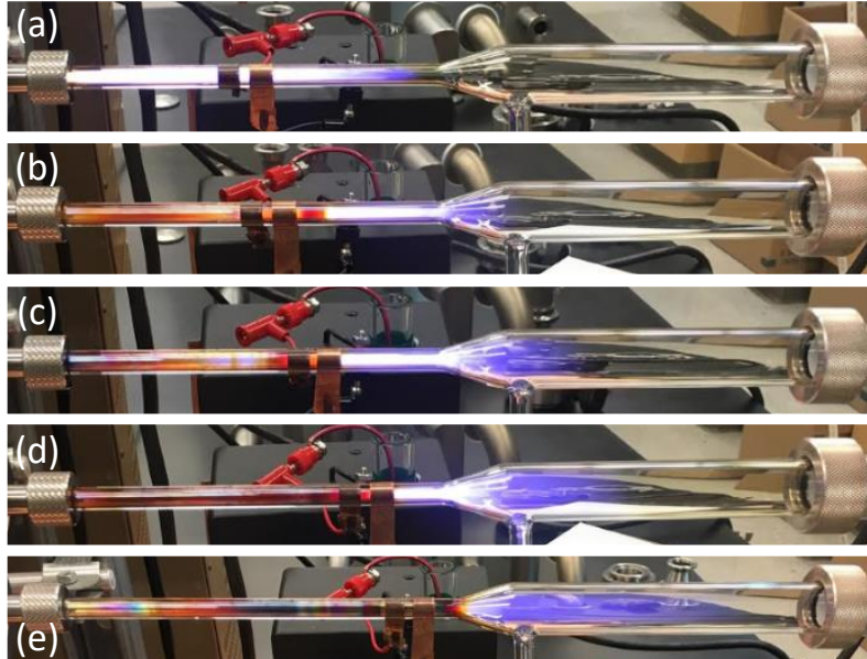
Figure 1.5. Plasma Effects from Electrode Spacing. These images show SiNCs synthesis with varying electrode placement. Similar plasma stretching can be induced with pressure, flows, and power level (each with different interactions and effects on SiNC size and quality). Note in a) we observed upstream arcing. Hydrogen was being injected in the sideports of these reactors, otherwise for e) (and possibly d)) we would likely have observed downstream arcing.
