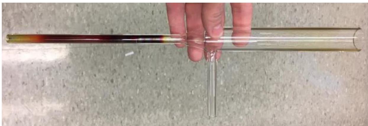
Figure 7.8. Typical Deposition on a Reactor Tube After 30-60 minutes of Synthesis.
