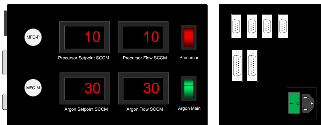
Figure 5.21. MFC Control Interface. This figure shows the front (left) and the relevant side (right) views of the MFC control interfaces. Two of these were constructed for our study, allowing for four independent gas flows (two for each interface). The DB15 connectors on the side view interface with the MFC. The DB9 connectors provide DC power to the pressure transducers (which have their own built in displays).
