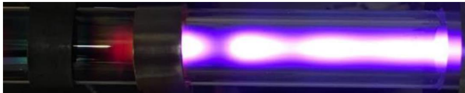
Figure 7.1. Striated Plasma Example. This figure shows the striated plasma for 60 sccm argon, 0.08 CHS (calculated), 30 watts, 0.31" I.D. straight reactor tube with the RF electrode 6 cm from the downstream disconnect.
