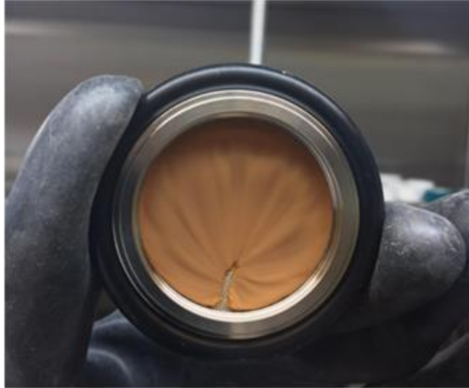
Figure 8.5. Successful Filter Collection for 900 nm SiNCs Using 72 Mesh Centering Ring.
