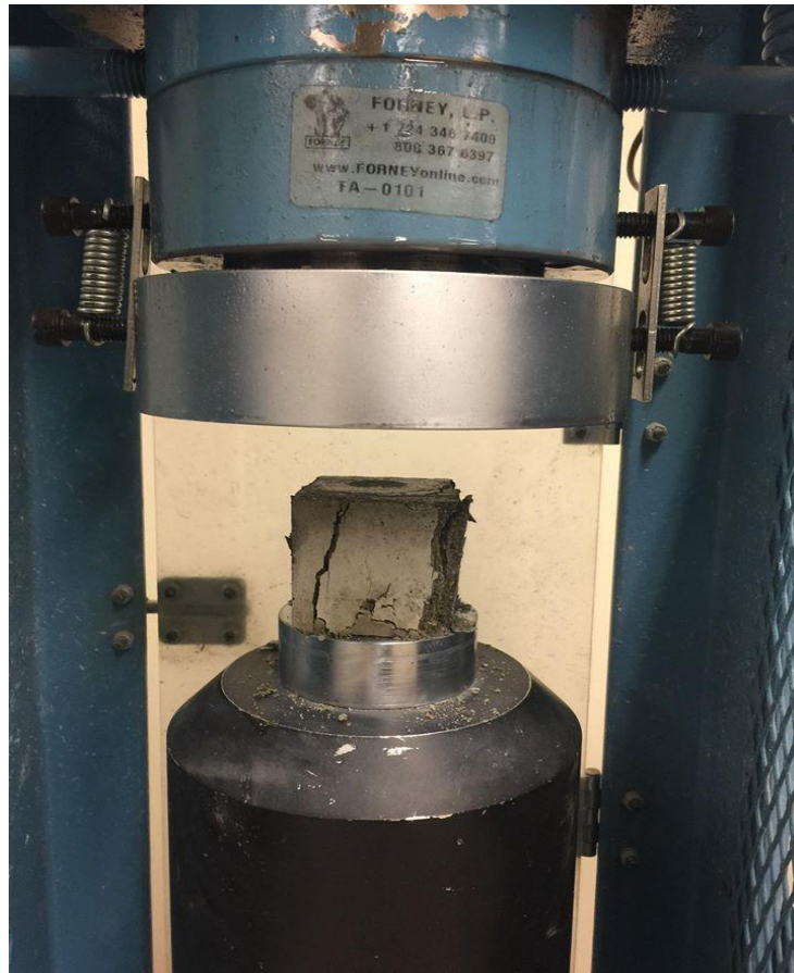
Figure 4.3. Failure of sample after application of load.
