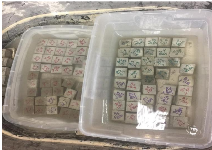
Figure 3.13. Cubes set for curing.
