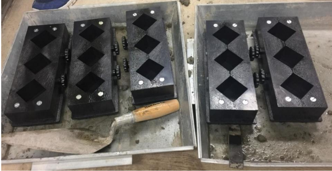
Figure 3.10. 51mm *51mm molds oiled and greased for casting of mortar cubes.
