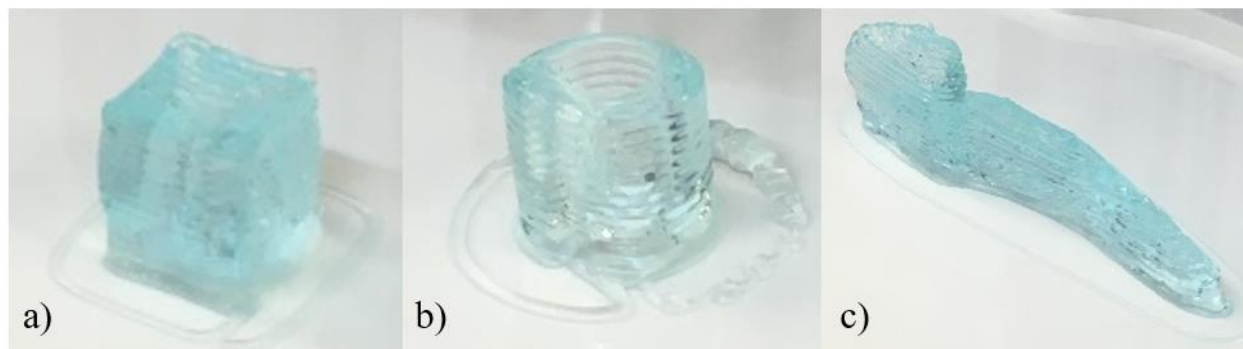
Figure 9. Different print geometries that were used to verify the printer parameters including a) a cube, b) a hollow cylinder, and c) a pancreas model.
