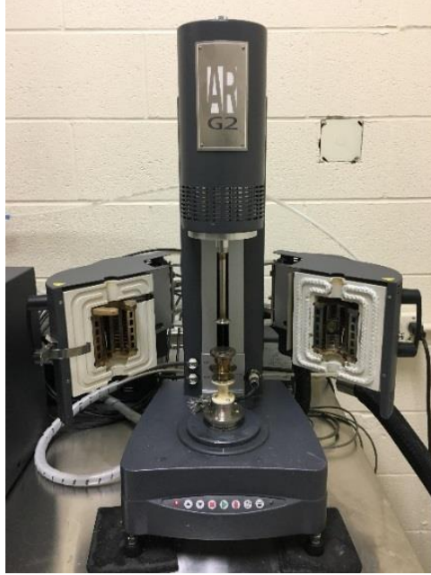
Figure 6. TA Instruments AR-G2 rheometer with parallel plate attachments used to perform rheological testing.
