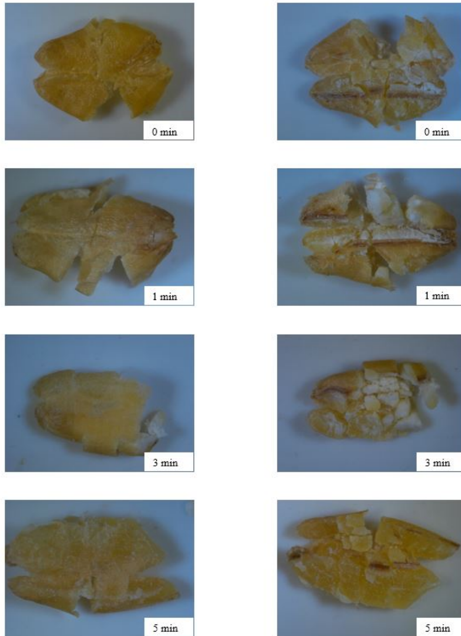
Figure 4. Effect of debranning time on the outer layer (left column) and inner layer (right column) views after debranned kernels passed through the first break roll.
