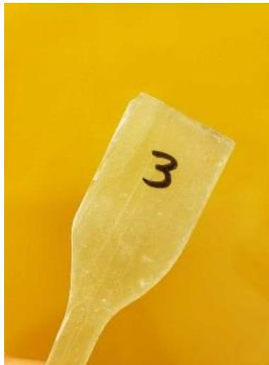
**Figure 3.8.** Cracking Observed with the DMESS Printed Formulations
