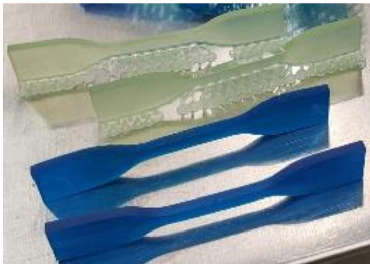
**Figure 3.7.** 0x Tensile Prints of MBSS with Supports and Moai Blue with Supports Removed
