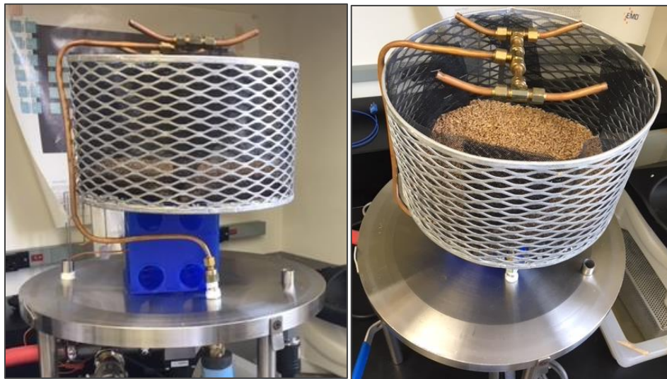
Figure 4. Pasteurization vessel arrangement in VSP.
