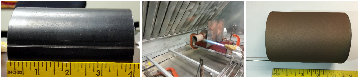
Figure 41. Pipe sample preparation and coating process.
