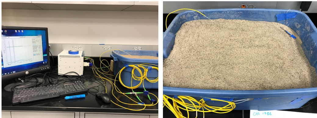
Figure 60. Experiment set-up for corrosion location detection.
