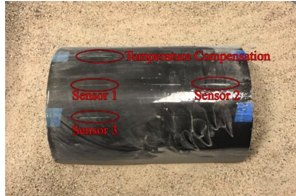
Figure 59. Steel pipe sample preparation for corrosion location detection.
