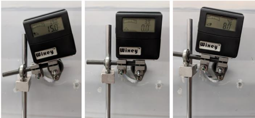
Figure 14. Testing the maximum range of motion of the actuator
