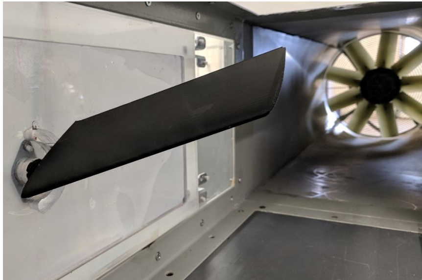
Figure 11. \Lambda = 27.6^\circ airfoil mounted in the wind tunnel
