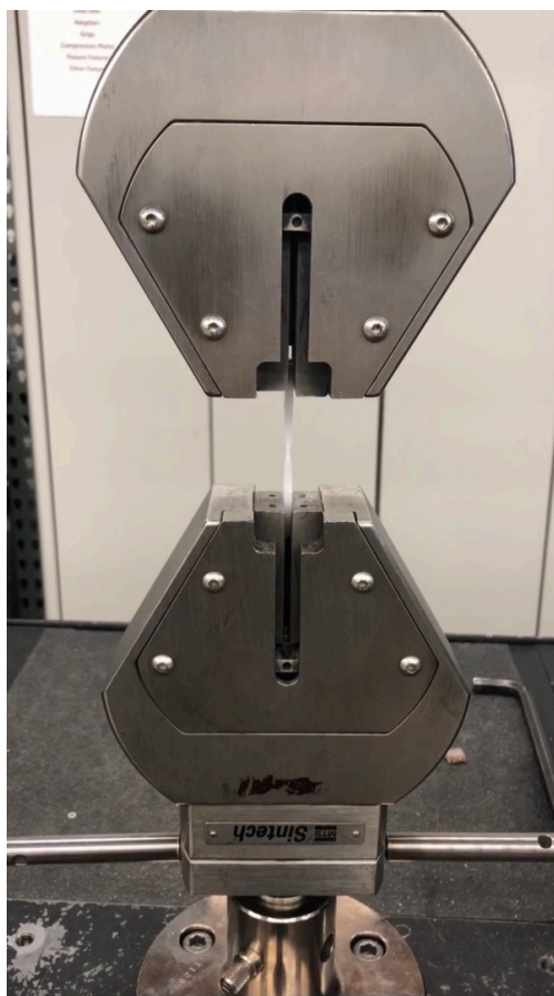
Figure 3.7. Tensile testing apparatus and the loaded sample.
