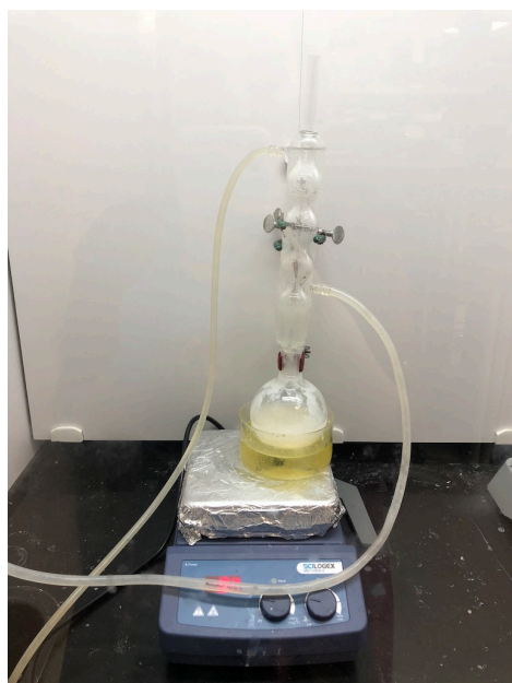
Figure 3.2. Solvent exchange process in the reflux condenser.
