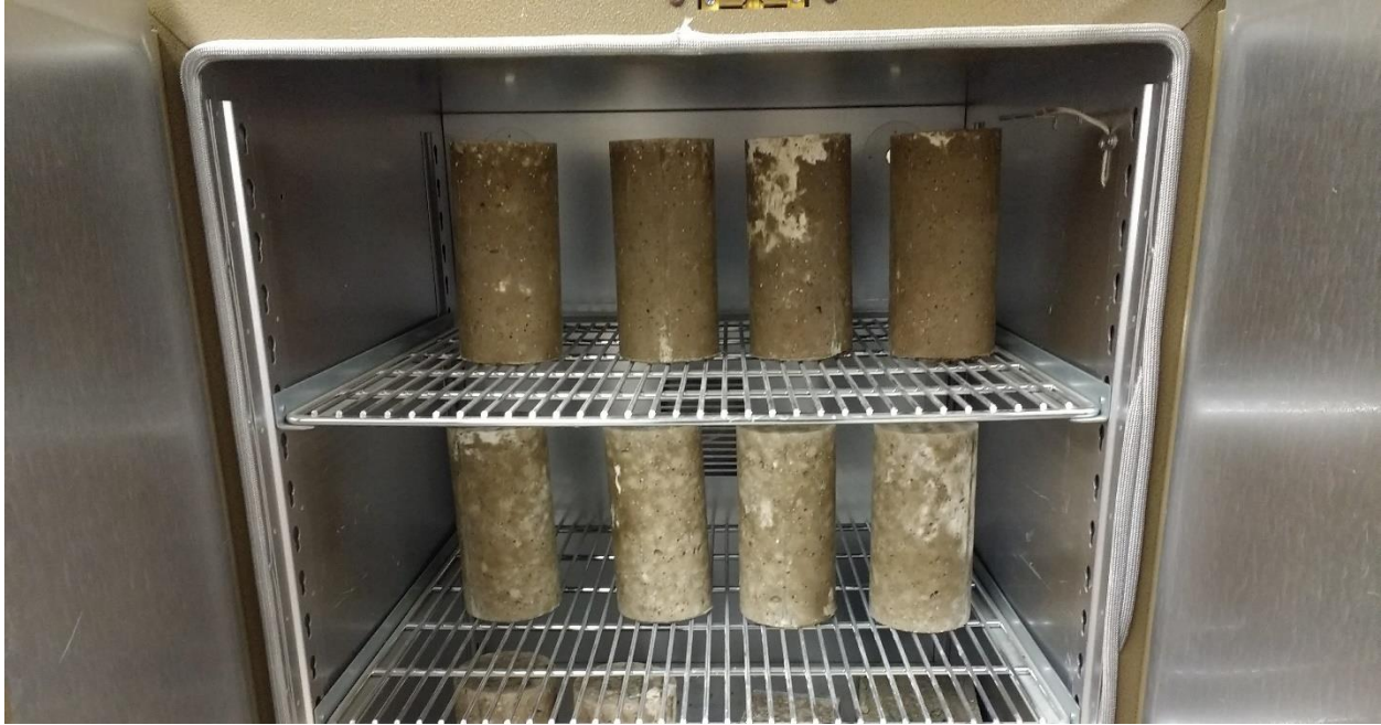
Figure 3.2. Oven curing of Geopolymer concrete samples
