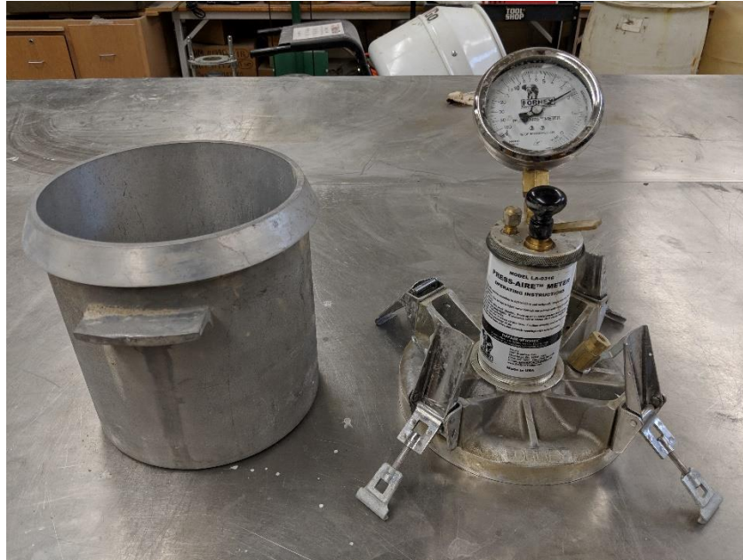
Figure 3.4. Concrete air meter
