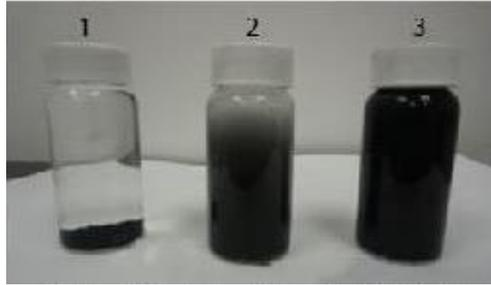
*Figure 8.* Comparisons of using the direct mixing, surfactant, and CMC surface treatment method (from left to right) of dispersing CNTs after two hours.
