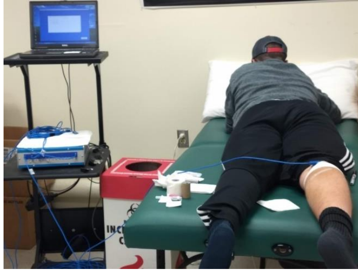
Figure A5. Thermocouple Secured to Leg and Plugged into 16-Lead Iso-Thermex Thermometer.
